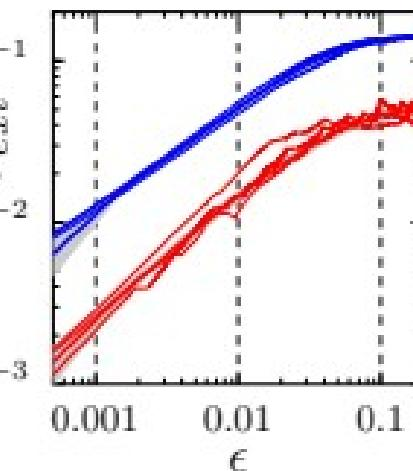
Strain-rate controlled loading:  $\sigma_{ext} = k[\dot{\epsilon}_a t - \epsilon(t)]$
