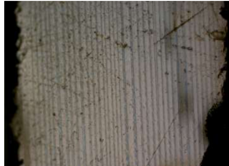
PMN-PT (001) (1-x)[\text{Pb}(\text{Mg}_{1/3}\text{Nb}_{2/3})\text{O}_3]-x[\text{PbTiO}_3] , x=0.32
